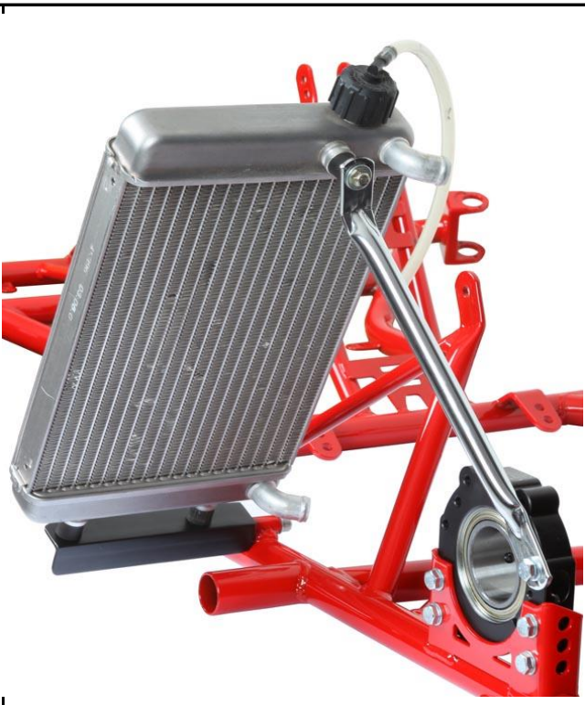
Foto of the frame from the side with the section of the supports for the radiator (radiator mounted)
